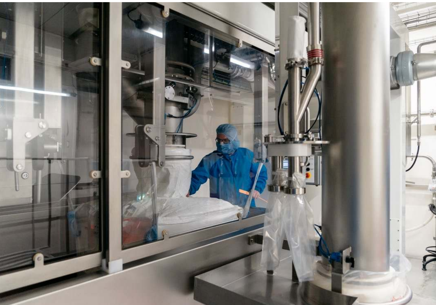
Lactose bagging in the Dry Mix plant 'Whey V' at the Leppersdorf site
