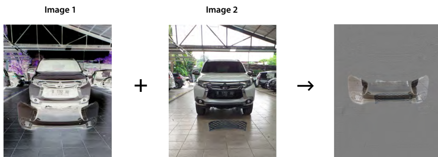
Example of fraud detection in accident images: An analysis by AI indicated that images 1 and 2 were derived from the same image and that the front part in each image has been deliberately doctored to disguise as being repaired.
