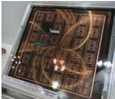
*510 x 515 mm panel chip-embedded interposer
