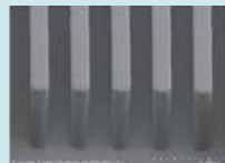
Resist pattern (resist line width 1.5 μm / wiring pitch 1.5 μm)
