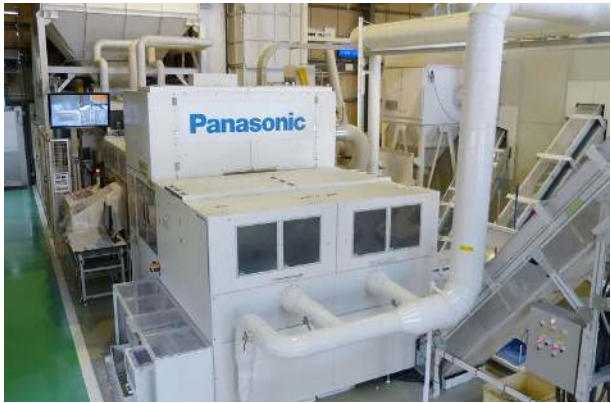
Near-infrared sorting machine that can sort three types of resin simultaneously
