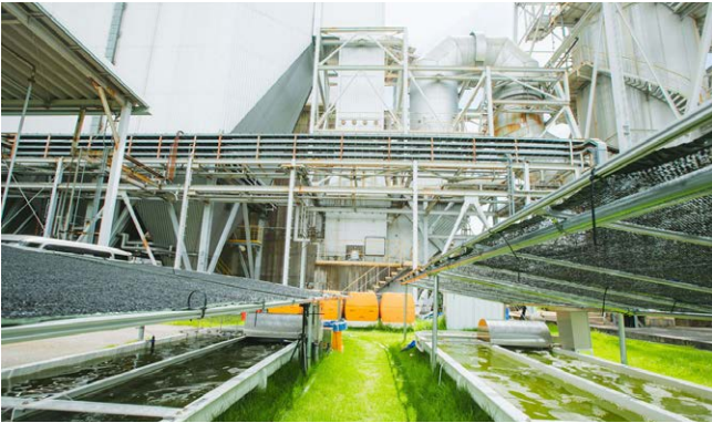
Microalgae cultivation test tanks set up next to the power plant at the Hiroshima Plant
