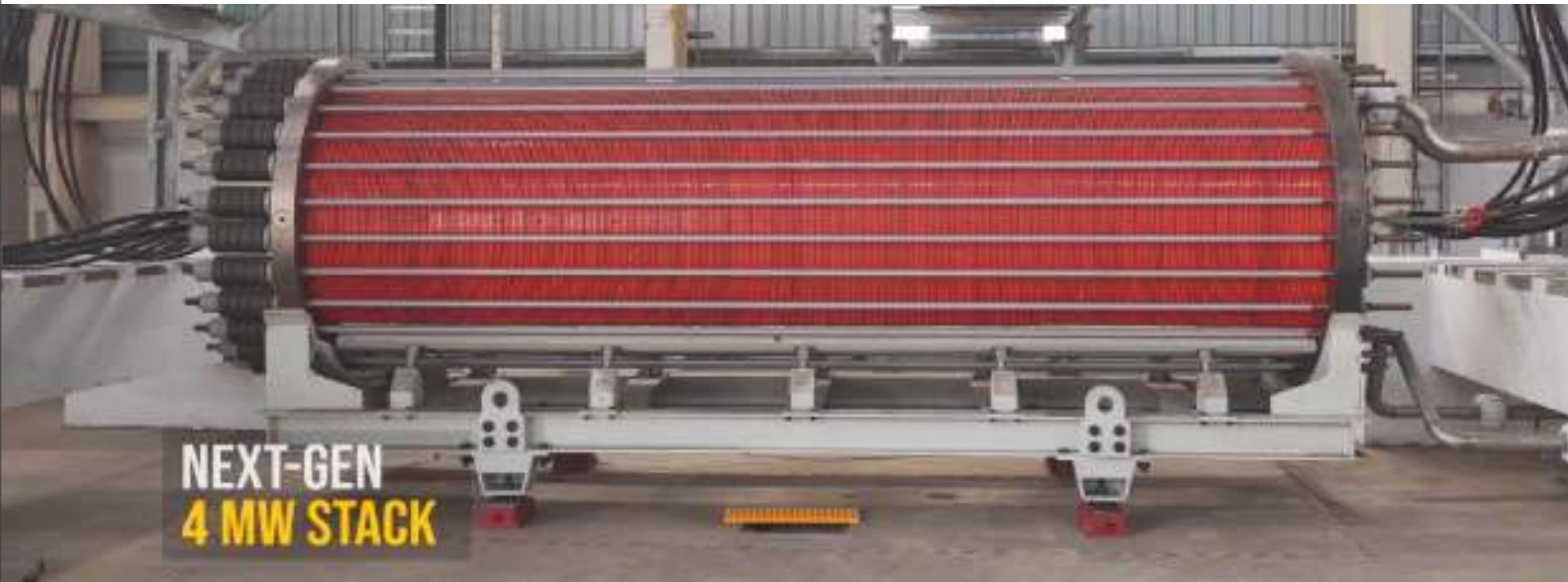
L&T's advanced pressurised alkaline electrolyser 4 MW XL Stack
