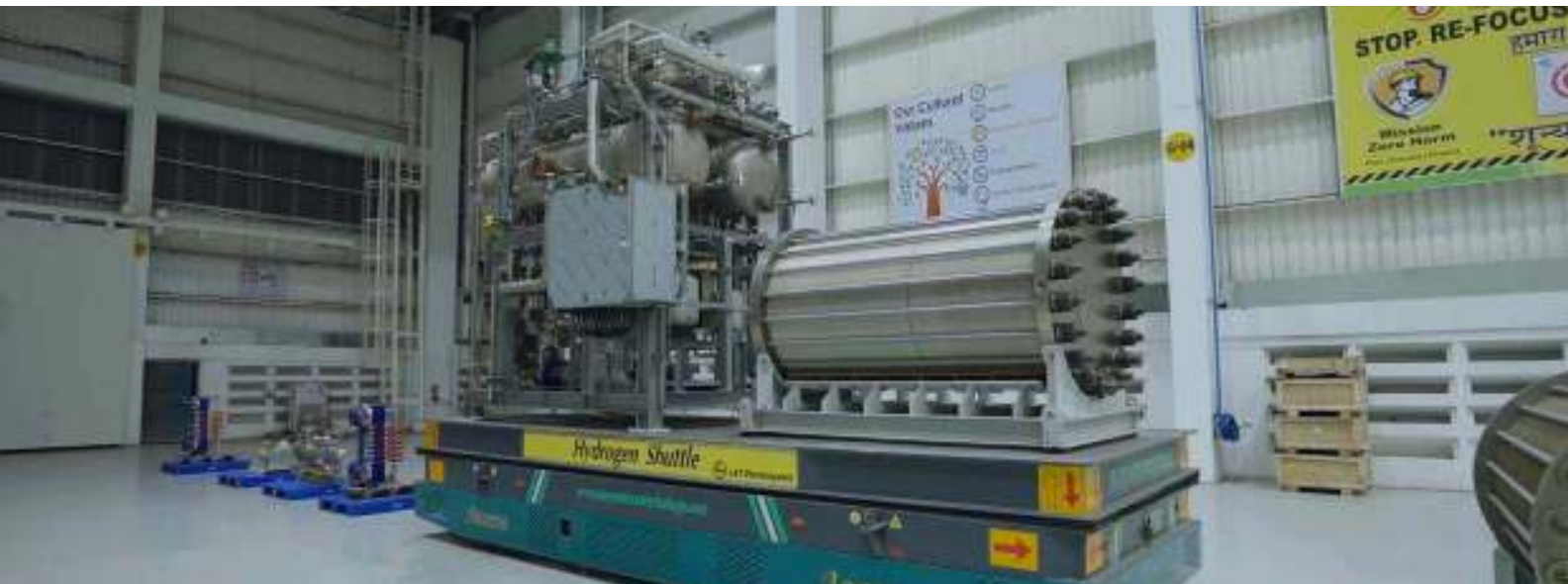
India's first indigenously developed Electrolyser at A. M. Naik Heavy Engineering Complex, Hazira, Gujarat
