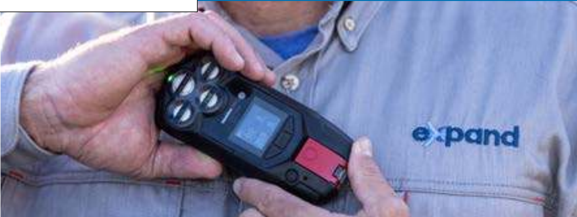
On-site personnel wear gas monitors as a hazard prevention tool. These monitors alert workers if air quality is compromised.
