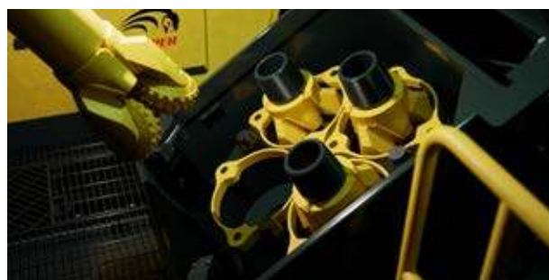
The Automatic Bit Changer (ABC) enables hands-free bit changes and enhances productivity and safety by eliminating human interaction with the drill string. Following the positive customer feedback from the introduction in the Pit Viper 270 series, Epiroc has extended the solution to the popular Pit Viper 351 blasthole drill rig.
