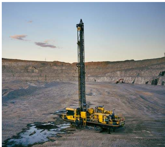
In October, Epiroc announced a large order for surface mining equipment in Australia from Newmont Corp., one of the world's leading gold producers. The rigs, among others the Pit Viper 231 rotary blasthole drill, will be operated tele-remotely, i.e. run with automation.
