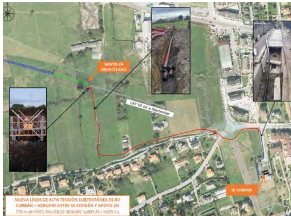
View of the different undergrounding points
