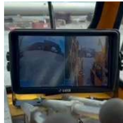
Cameras are mounted at blind spots with a monitor in the cab for the driver to see.
