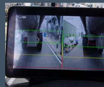
Proximity protection technology alerts drivers to the presence of pedestrians. Different types of technology are being implemented at Dow sites around the world.
