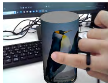
Touching a tangible object onto which the image of a bird has been superimposed in the AR space. The tactile sample developed by DIC allows the reproduction of a highly realistic texture. (This photograph was taken at Saitama University's Komuro Laboratory.)
