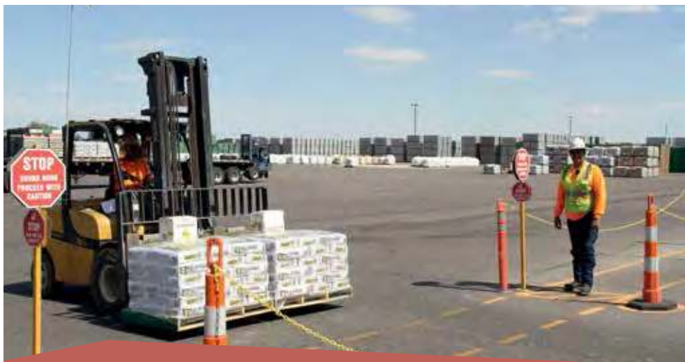
Vehicle-pedestrian segregation is a focus across the CRH Group to reduce the risk of accidents from mobile plant movements. At the Superlite Lone Butte location in Chandler, Arizona, US, designated walkways, signs and barriers are employed in a custom-designed system to ensure the safety of pedestrians.
