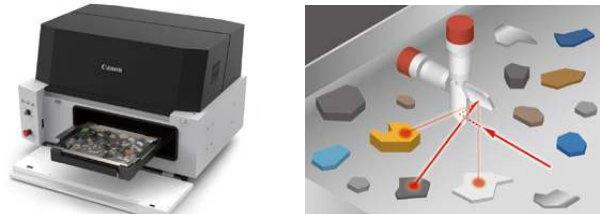
(Left) Raman Plastic Analyzer TR-A100 (Right) Canon's high-precision galvanometer scanner sequentially irradiates multiple plastic pieces arranged on a tray with a laser, and the material is identified by spectroscopically analyzing the material-specific Raman scattered light generated in the process.
