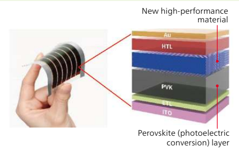
(L) Perovskite solar cell (R) Structure of perovskite solar cell with newly developed high-performance material
