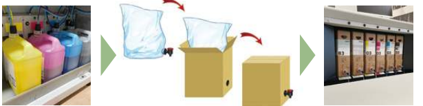
Mechanism of the Bag-in-box System
