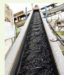
Recycled toner pellets used as asphalt additive
