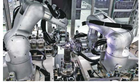
Automated production process for interchangeable lenses
