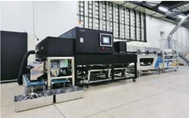
High-precision sorting equipment capable of measuring black plastic pieces, which are difficult to identify
