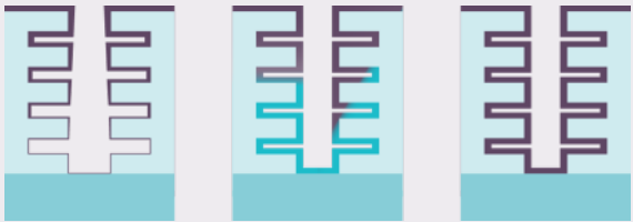
(1) Step coverage not OK (2) Step coverage OK, but properties not OK (3) Step coverage, composition, and properties all OK
