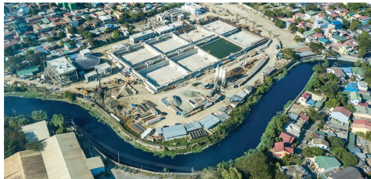
Manila Water's pipelaying project in Ilugin, Pasig is close to completion will be the largest Sewage Treatment Plant in the country with a capacity of more than 100 million liters of used water per day.
