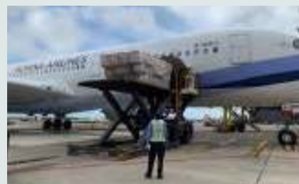
Ramp Loading and Unloading Operations
