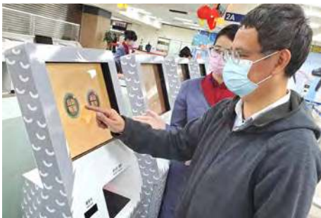
It Uses a 19" Infrared Non-Contact Touch Screen that Allows The User to Complete All Check-in Procedures by Hovering Their Fingers Over the Screen Instead of Touching it
